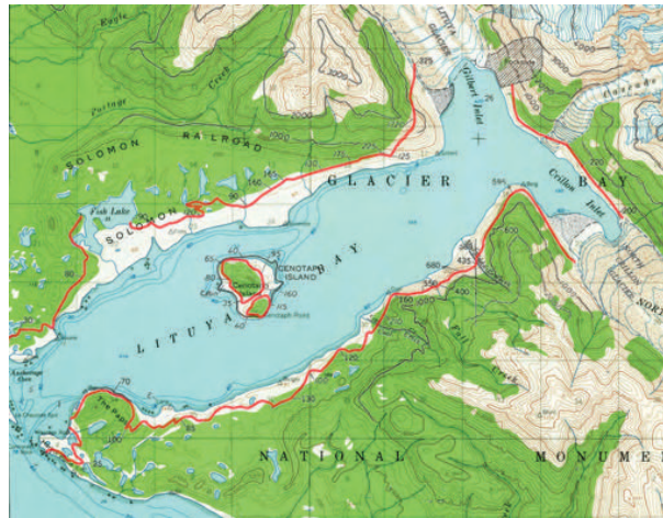
Figure 1. Topographic map of Lituya Bay (U.S. Geologic Survey, 1961) showing the settings and trimline of 1958 megatsunami (based on data from (Miller, 1960)). Units in feet.
