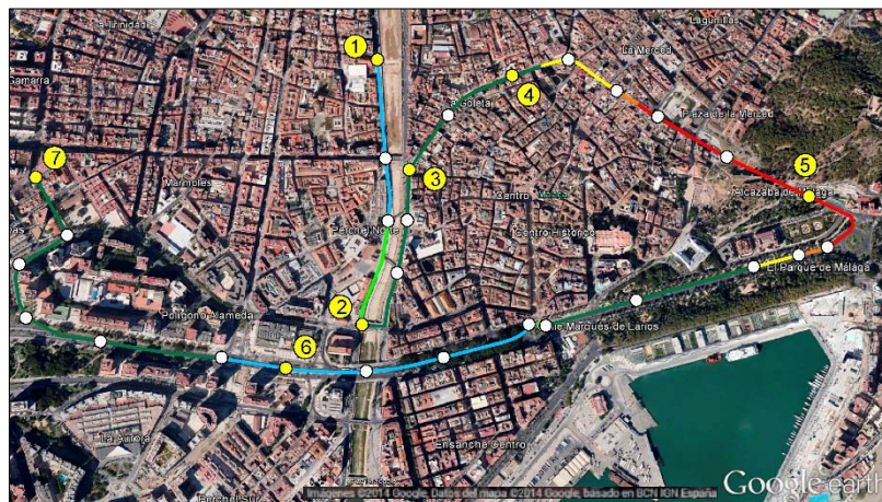
Maps created with the mobile node. Light colors represent low traffic intensities and dark colors high traffic intensities.
