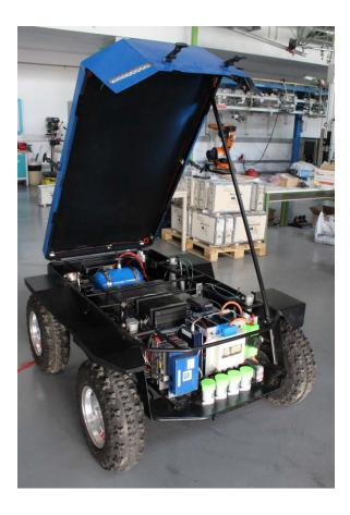
RAMBLER used in-wheel brushless motors. Each motors are controlled by an embedded board that integrates a microcontroller (µC) and an independent H-bridge power stages.
