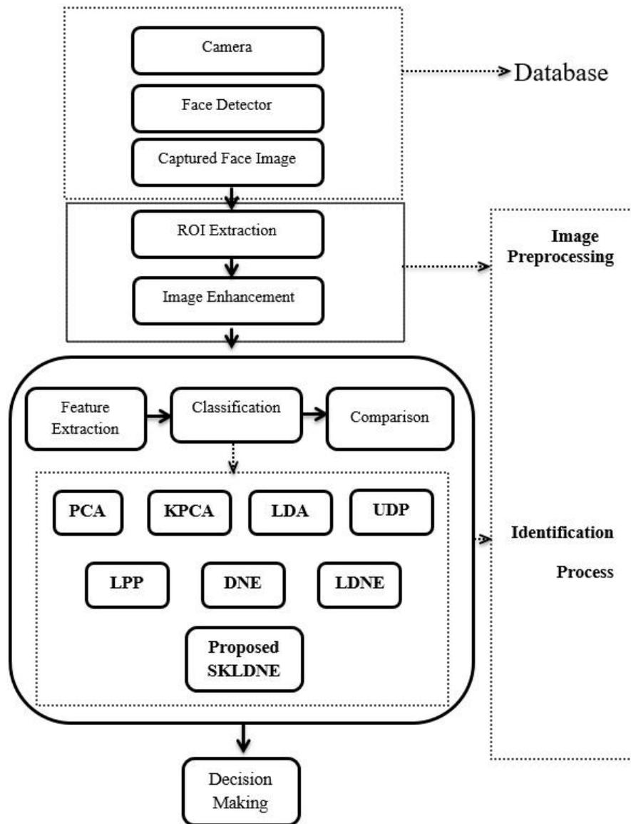
Figure 3.3. The overall view of main recognition algorithm
