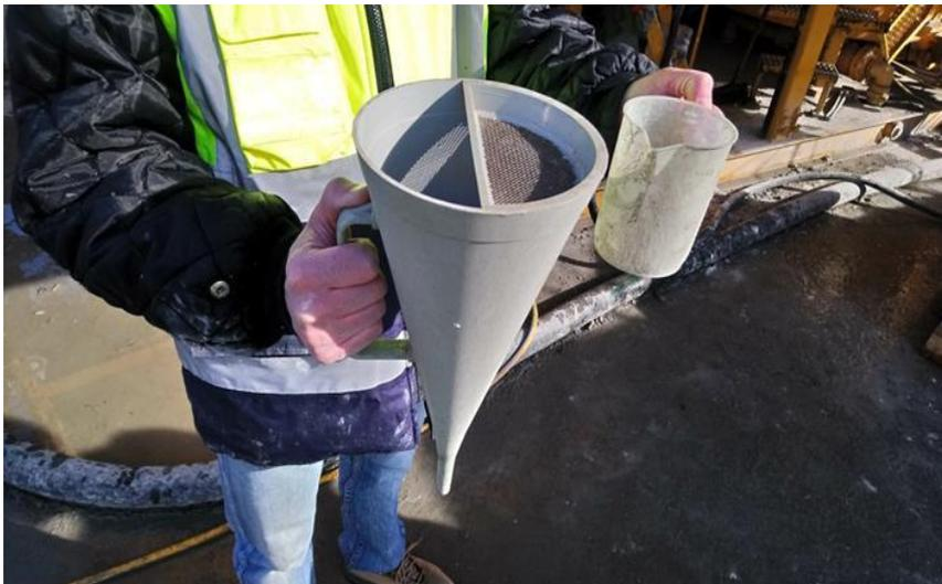
FIGURA 6. 4: ENSAYO CONO DE MARSH
