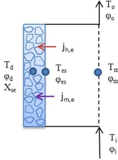
Figure 3. Heat and mass flows in a control volume.
