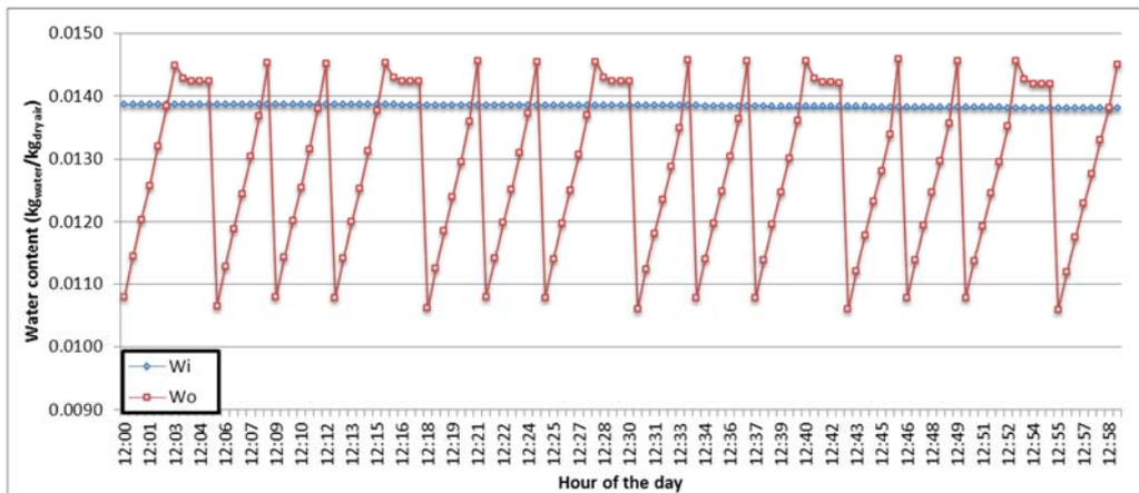
Figure 4. Air humidity variations in the desiccant channel.
