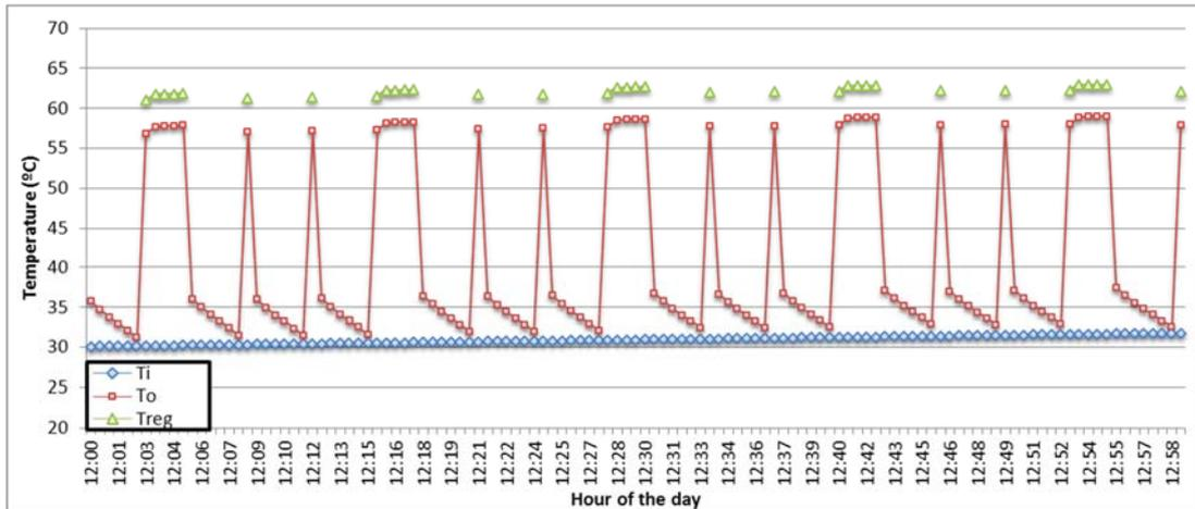
Figure 5. Temperature variations in the desiccant channel.
