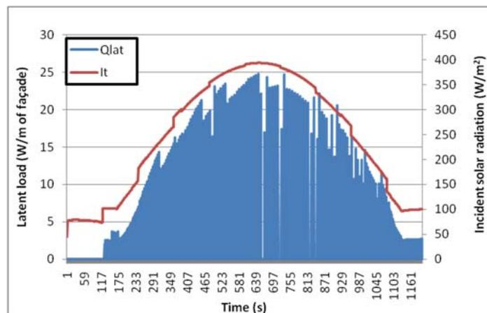
Figure 6. Incident solar radiation and latent load removed by the façade.
