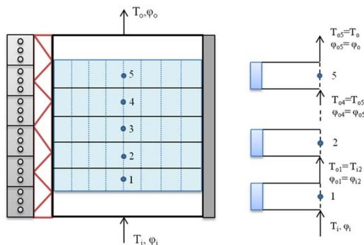
Figure 2. Vertical discretization of the desiccant domain.
