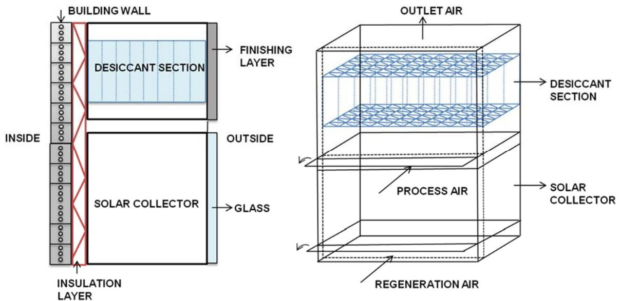
Figure 1. Schemes of the desiccant façade. a) Layers from inside to outside. b) Operation modes
